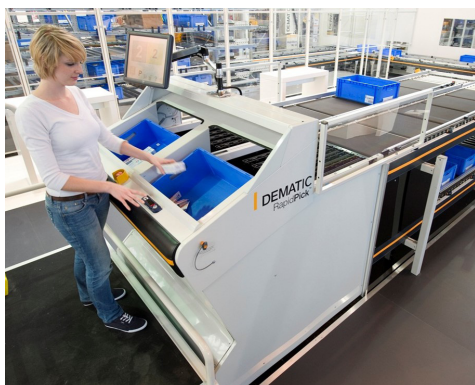
RapidStore : Station de picking "Goods-to-person" (Dematic)
